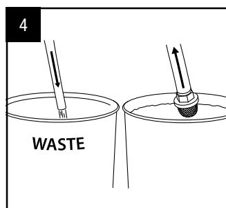
Allow fluid to flow out of prime tube
