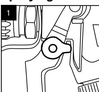
Put trigger safety lever in locked
