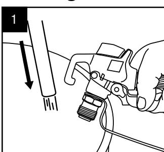
Submerge suction tube in paint. Turn Power Switch ON, and trigger gun into waste pail. When paint comes out of return tube, turn Prime/Spray valve to SPRAY. When paint comes out of gun, release trigger. Pump will build up pressure and motor will stop.
