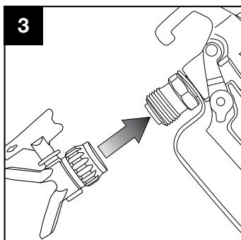
Insert Saddle Seat first into Spray Guard, as shown, with the curved part of the Saddle aligned with the Spray Tip hole. Use the plastic pointer on the Spray tip to fully seat, if needed.
