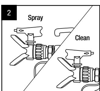
Install tip and guard on gun and hand
